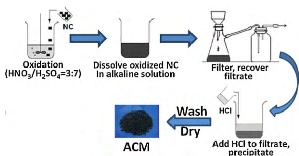
Fig. 1. Schematic flow chart for the ACM preparation.
